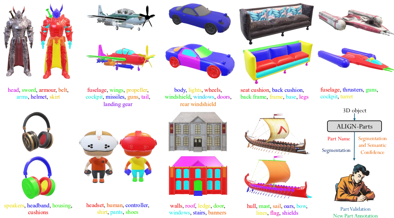
Figure 12: TexParts Dataset. We demonstrate human-in-the-loop annotation of Texverse [Zhang et al. 2025] using ALIGN-Parts, enabling scalable dense 3D part segmentation.
